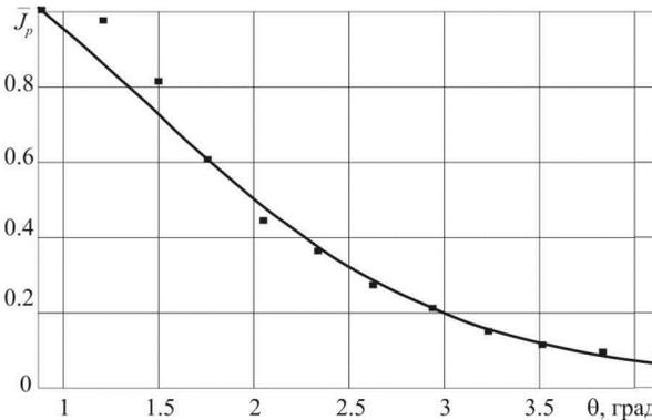
**Figure 4.** Experimental (points) and calculated (solid line) of the scattering indicatrix for polydisperse aerosol droplets in the ejection nozzle spray pattern.
