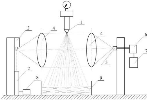
**Figure 3.** The experimental facility layout for the implementation of spectral transmittance method: 1 - nozzle; 2 - laser; 3 - mechanical system; 4 - optical system; 5 - photodetector; 6 - oscilloscope; 7 - personal computer; 8 - generator unit; 9 - receiving tank.
