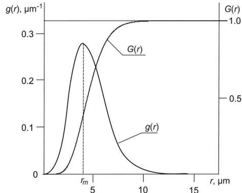
**Figure 5.** The differential and integral functions of mass droplets size distribution.
