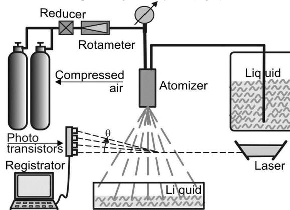
Figure 1. Pneumohydraulic stand with optical diagnostics system.
