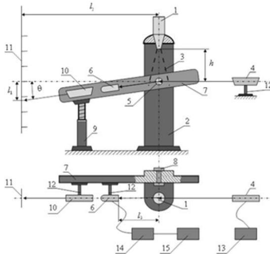
**Figure 2.** The experimental facility layout for the implementation of method of small-angle scattering indicatrix.
