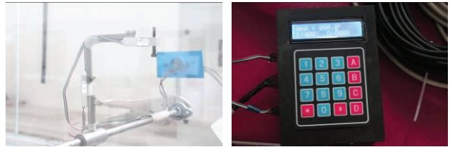
Figure 3. Automatic computer controlled force measurement system.
