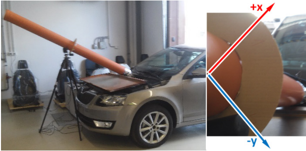
Figure 1. Experimental setup. On the left: Stilling channel during measurements. On the right: the ring around the cross-section area of tube where the probes were placed (axis location +x=45^\circ +y=135^\circ from the horizontal plane).
