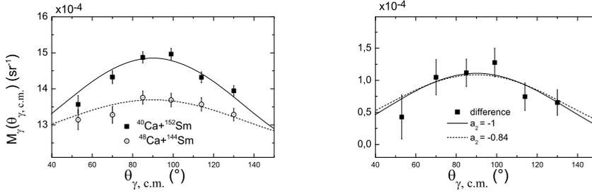
Figure 2: Center-of mass angular distribution of the evaporation  $\gamma$ -rays for the two reactions (left) and of their difference (right) in the energy range 9-15 MeV corrected by the experimental setup efficiency. The lines are described in the text.
