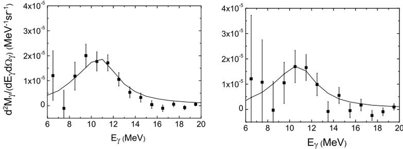
Figure 1: Difference between the charge asymmetric and charge symmetric reaction bremsstrahlung-subtracted center-of-mass  $\gamma$ -ray spectra for fusion-evaporation (left) and fission (right) events. The lines are described in the text.
