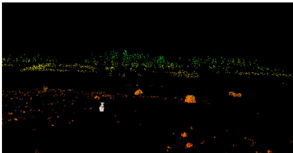
Figure 10: Ground segmented out, leaving only above ground objects.
