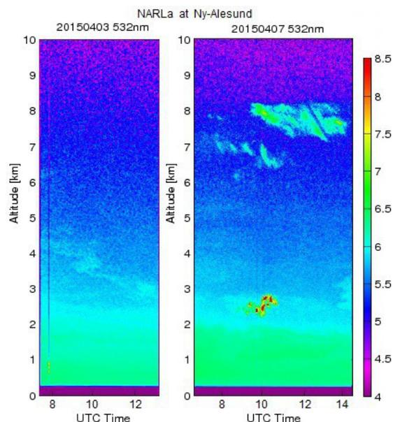
Fig.4: Attenuated backscattering coefficient profiles at 532 nm [1/m/sr] measured by NARLa on 03/04/2015 and 07/04/2015 in Ny-Alesund, Arctic. The signals are available for evaluation in the range between about 300m up to 10km. Quick-looks of the data set are given at <http://www.polandaod.pl>.
