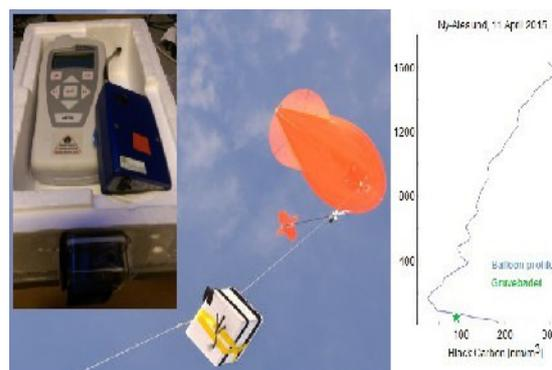
Fig.3: The iCAP set installed on tethered balloon for absorbing particles profiling. On the right an ascent with black carbon measurement taken at Ny-Alesund on 11/04/2015 compared with in-situ measurement at Grubebadet station.
