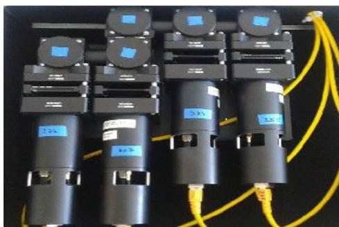
Fig.1: The NARLa detector unit consisting of elastic and Raman channels at 355nm and 532nm.
