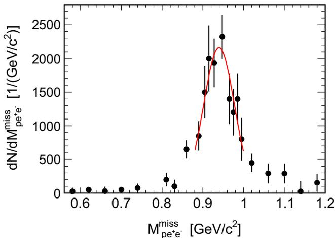
**Figure 1.** Missing mass distributions for the  $p, e^+e^-$  events, with dielectron mass larger than  $150 \text{ MeV}/c^2$ . The experimental data distribution (black dots) was fitted with a Gaussian distribution (red line).
