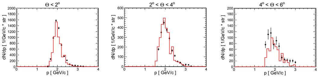
**Figure 2.** Momentum distributions of the spectator measured by time of flight in FW. Experimental data (black dots) are compared to the simulation (red solid line) for the indicated emission angles and dielectron pairs with  $M_{e^+e^-} < 0.14 \text{ GeV}/c^2$ . Simulated spectra are scaled to the same global experimental yield.
