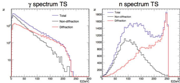
**Figure 4.** Expected spectra of photons (left) and neutrons (right) around  $0^\circ$  using PYTHIA 8212. Red and black histograms show the spectra originated from the diffractive and non-diffractive processes while purple show the total inclusive spectra.
