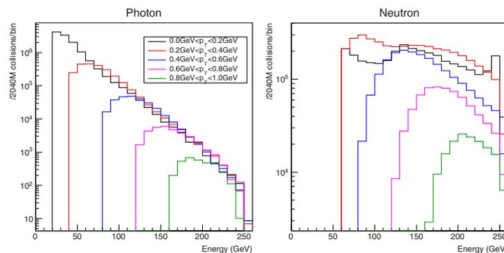
**Figure 2.** Expected observed spectra of single photon (left) and neutron (right) events after 12 hours of data taking. Data acquisition efficiency is taken into account, but the resolution is not considered.
