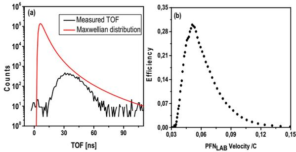
**Figure 5.** (a) Comparison of measured TOF with Maxwell distribution ( $kT=1.31$  MeV, flight path=65 cm,  $12 < TOF < 75$  [ns],  $0.37 < E_n < 11$  [MeV]) that was used to calculate the ND efficiency dependence on the PFN velocity (b).
