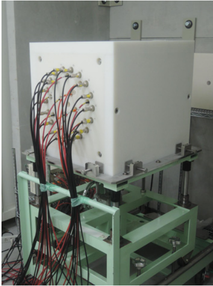
Figure 8. A flat-efficiency neutron detector.
