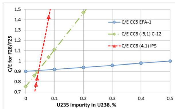
**Figure 3.** C/E for F28/F25 depending of the U-235 content in the U-238 deposit of the FC. The calculated results obtained with MCNP and JEFF-3.1 data were used.
