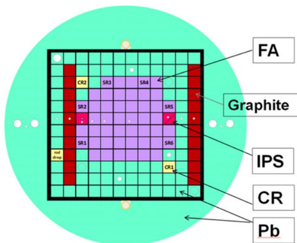
**Figure 1.** VENUS-F CC8 core to simulate reflector and IPS of MYRRHA.
