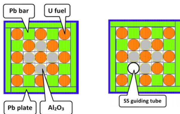
**Figure 2.** Left: fuel assembly; Right: experimental fuel assembly.
