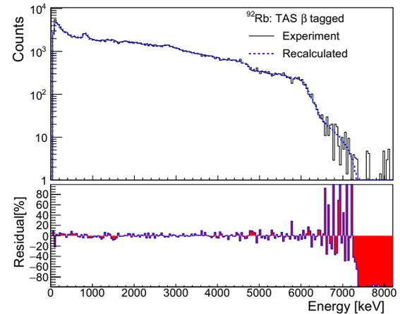
**Figure 1.** Upper panel: comparison between measured spectrum (black continuous line) and reconstructed one (blue dashed line) with the feeding obtained from the TAGS data analysis. Lower panel: residues between the two curves reported in the upper panel.
