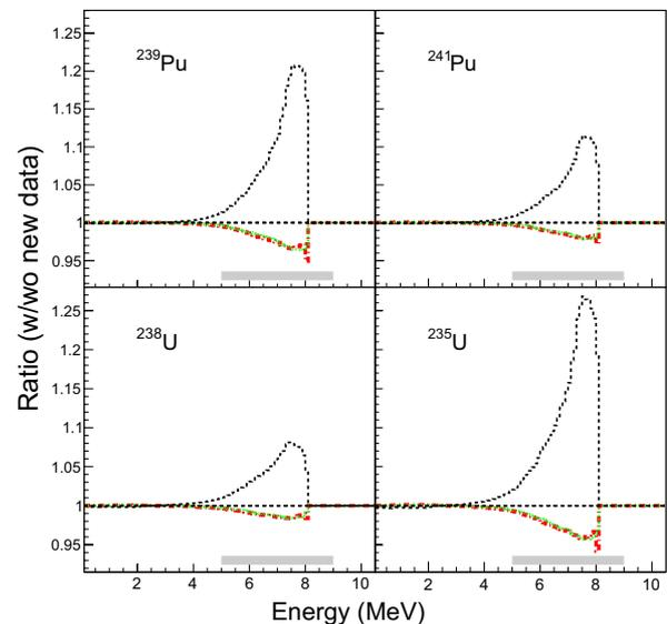
**Figure 2.** Ratio between the antineutrino spectra calculated using the latest TAGS results with respect to the data on  $^{92}\text{Rb}$  decay used in [4] (thick red dashed-dotted line), in [20] (green dotted line) and in [17] (black dashed line). The sharp drop in the ratio, in one single bin located at the Q value of the  $^{92}\text{Rb}$ , is due to the different values in Q given in [27] and *ENSDF*, that were used to reconstruct the antineutrino spectrum.
