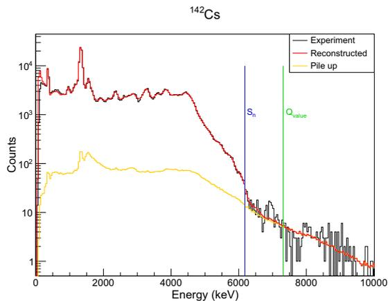
**Figure 3.**  $^{142}\text{Cs}$ : comparison between measured spectrum (black continuous line) and reconstructed one (red continuous line) with the feeding obtained from the TAGS data analysis. The contribution of pile-up signals is shown (yellow line).
