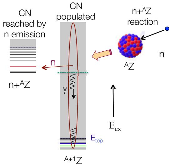
**Figure 1.** Schematic of a capture reaction. In a compound neutron capture process, the neutron and target nucleus  ${}^AZ$  fuse to form the compound nucleus  ${}^{A+1}Z$ , which subsequently decays via a  $\gamma$ -ray cascade. This occurs in competition with neutron emission (shown) and other decays (not indicated).
