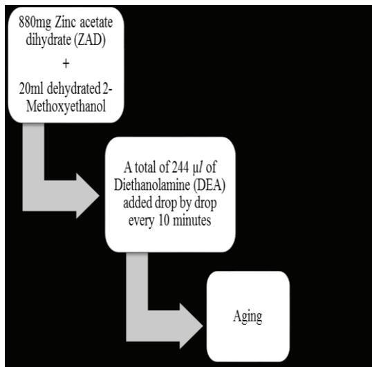
Fig. 3. Steps for ZnO Sol-gel preparation.
