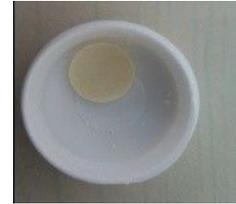
Fig. 1. Undoped ZnO pellet
