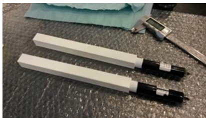
Fig. 8. Two units of the PADME ECAL detector. They consist of a BGO crystal ( 10 \times 10 \times 230 \text{ mm}^3 ) glued to a 19 mm diameter photomultiplier.
