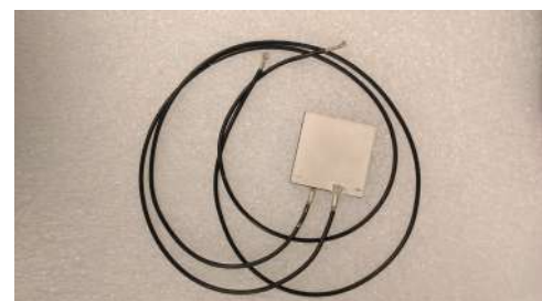
Fig. 14: PZT plate with commercial electrodes, epoxied ring terminals and wiring.
