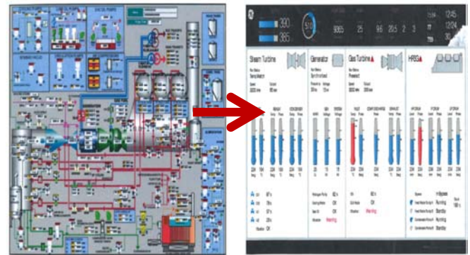
Fig.2. An example of resulting plant overview screen
