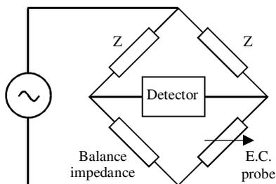
Fig. 9. Simplified impedance bridge circuit used for simulations. The balance impedance is a replicate of the eddy-current probe, but it is held at static conditions over a test sample.
