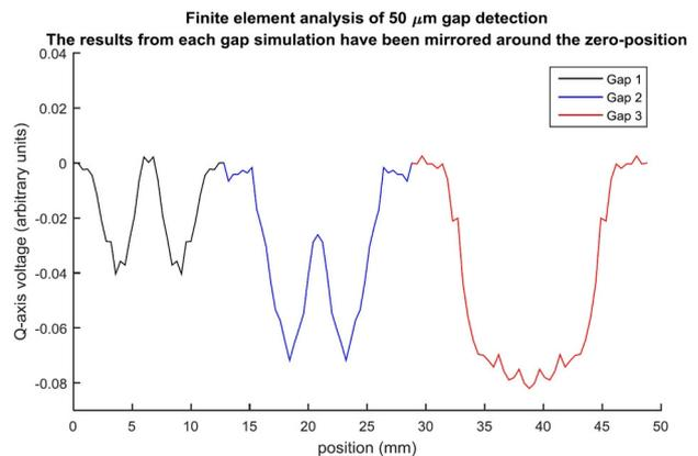
Fig. 19. Gap response vs. position. The results from the three simulations have been arranged in sequence. The three signal responses are in the same scale.
