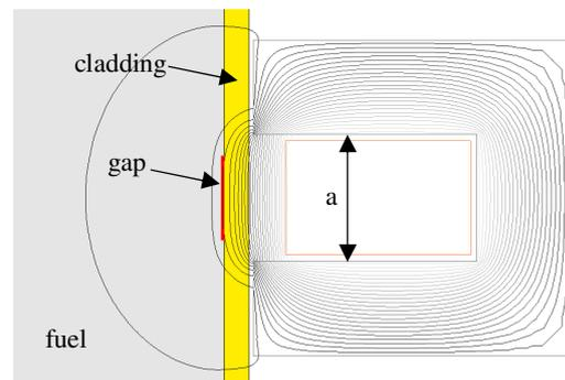
Fig. 10. Screenshot from a 2D FEM-study investigating the magnetic field penetration as a function of core slot-opening  $a$ . The simulations were performed at 250 kHz.
