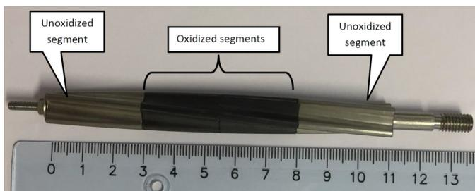
Fig. 6. Photo of the dummy rod used for testing oxide thickness measurements in the mock-up of the measurement station.
