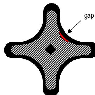
Fig. 7. Cross-section of fuel rod with gap indicated. The gap is shown in red.
