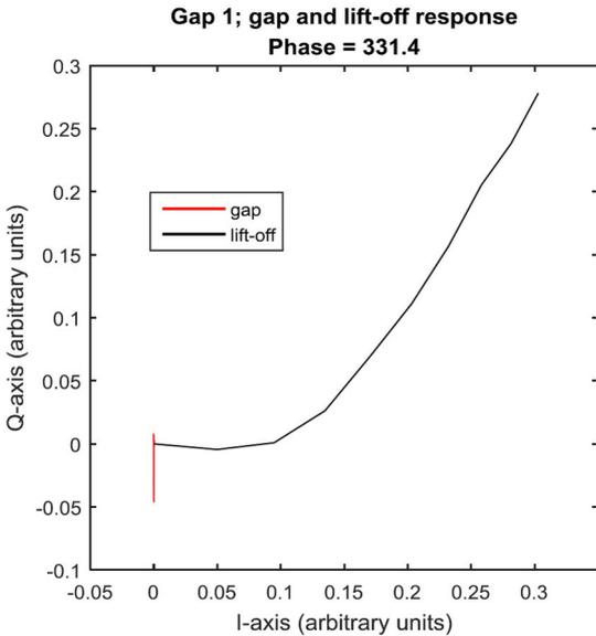
Fig. 16. Gap and lift-off response to simulated gap 1. The gap response is plotted in red, while the lift-off response is plotted in black.
