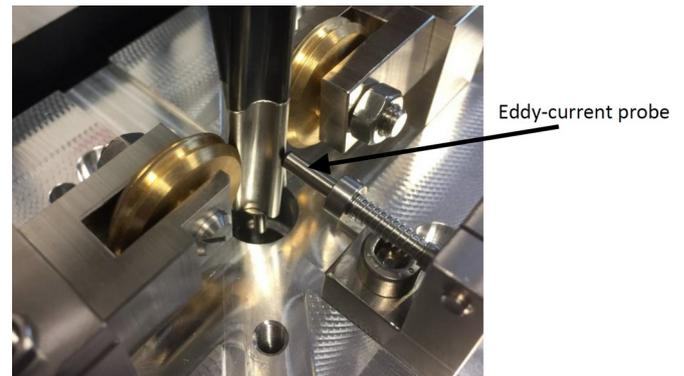
Fig. 5. Eddy-current probe for oxide thickness measurements mounted in mock-up test station together with a fuel rod dummy.
