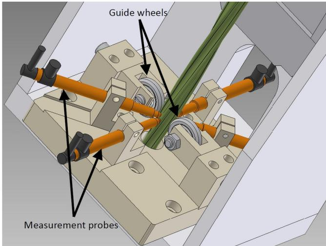
Fig. 3. Schematic conceptual view of the measurement station.
