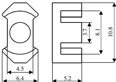
Fig. 12. Main dimensions of core. All dimensions are given in millimeters.
