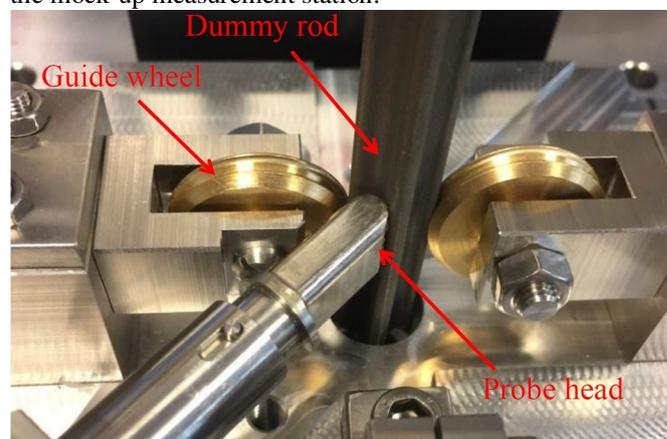
Fig. 23. Close-up of dummy fuel rod and gap-detection probe in measurement station mock-up.
