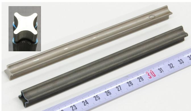
Fig. 20. Parts of dummy rod for eddy-current gap detection tests. The upper part represents the fuel, with small gaps machined onto the surface. The gaps shown are oval, whereas the opposite side is equipped with rectangular gaps. The lower part represents the cladding. The inset shows the assembled dummy rod. The dummy rod is not helically shaped.
