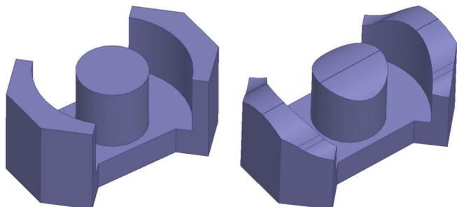
Fig. 11. Core before (left) and after (right) modification.
