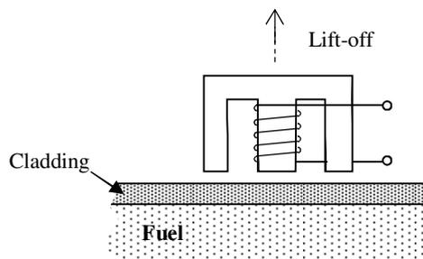
Fig. 15. Lift-off. The probe is removed from the surface of the fuel cladding
