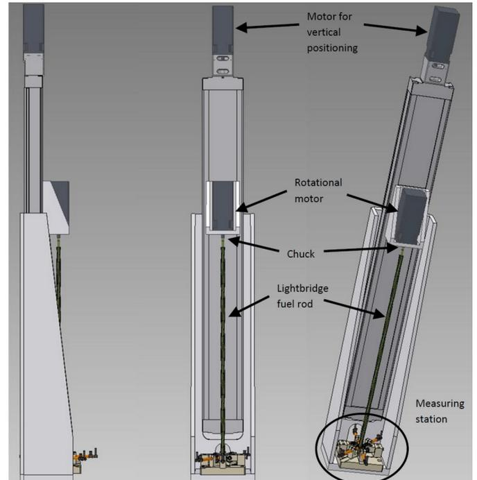
Fig. 2. Lightbridge measurement station. The encircled area in the lower right corner is shown in detail in Fig. 3.
