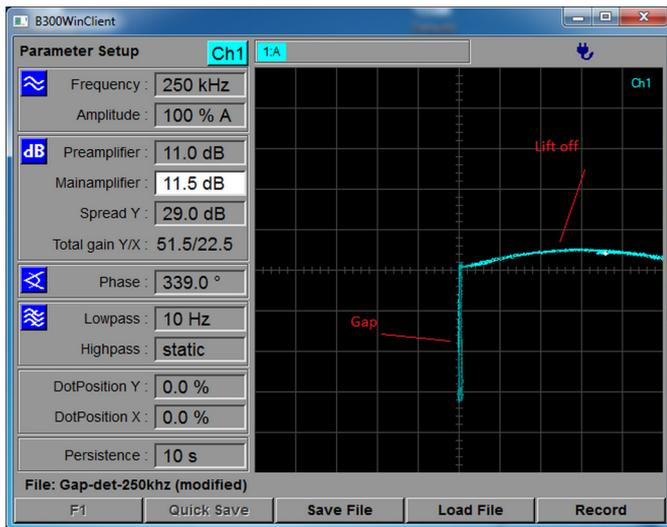
Fig. 24. Gap and lift-off response. The gap-response is obtained from scanning a 50  $\mu\text{m}$  deep 4 x 4 mm rectangular gap.
