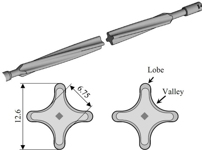
Fig. 1. Lightbridge metallic fuel rod with cross sections showing the characteristic, cruciform design. The Zirconium-alloy cladding is metallicly bonded to the Uranium-Zirconium fuel core. The central displacer (diamond in the center) consists of Zirconium or a Zirconium alloy containing burnable neutron absorbers.
