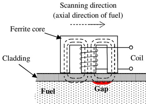
Fig. 8. Schematic illustration of a single-coil eddy-current probe scanning over a gap between fuel and cladding.
