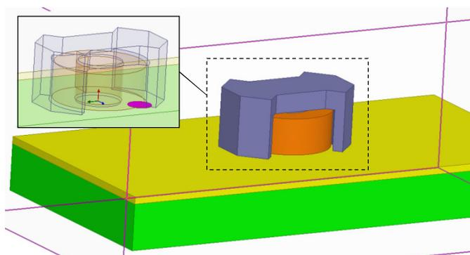
Fig. 13. FEM-model of probe. Picture inset at top left corner shows the gap in purple, located under the cladding layer.
