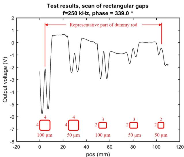
Fig. 25. Test results from gap-detection scan on the side of the dummy rod with rectangular gaps. The dimensions (in millimeters) and depth of each gap is included in the figure.
