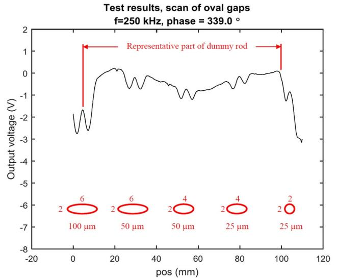
Fig. 26. Test results from gap-detection scan on the side of the dummy rod with oval gaps. The dimensions (in millimeters) and depth of each gap is included in the figure.
