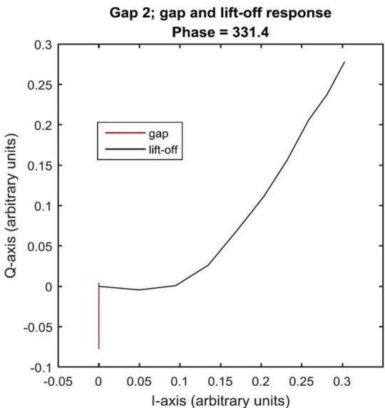
Fig. 17. Gap and lift-off response to simulated gap 2. The gap response is plotted in red, while the lift-off response is plotted in black.
