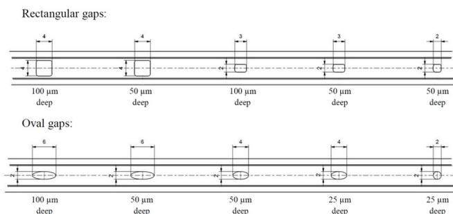
Fig. 21. Gap geometry with dimensions on the two opposite sides of the dummy rod. The same gap-geometry is reproduced in Figs. 25 and 26.
