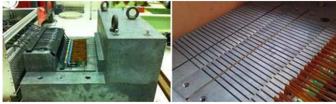
Fig. 1. Multi-CdTe detector, with the collimators [3].
