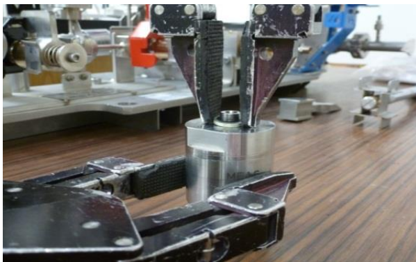
Fig. 2. Pressure gauge seal replacement by remote-handling
