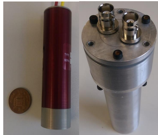
Figure 4 The CeBr 3 inorganic scintillator detector without and with aluminium casing.
