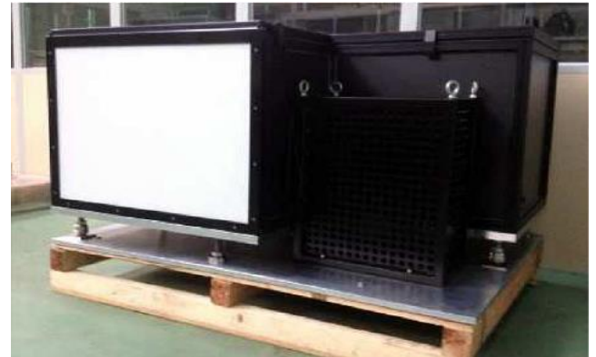
Fig. 5. 2D scintillator detector. The scintillator screen is imaged by a low noise camera through a 45° tilted mirror. The screen size is 80 x 60 cm 2 .
