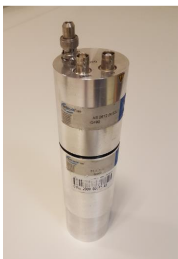
Figure 3: 2x2 inch LaBr 3 scintillator.
