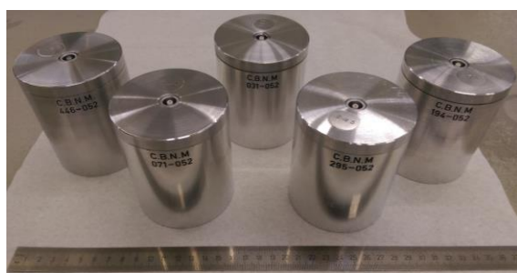
Figure 7: Uranium certified standards.
