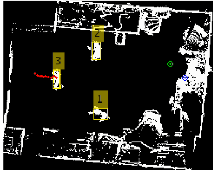
Fig. 5. Top-Down frame of LiDAR data showing the Kalman filter tracking of three persons. Person 3 is carrying the radioactive material and is given a red track.
