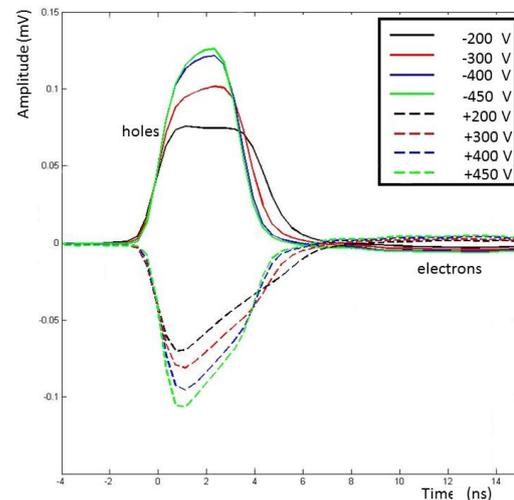
Fig. 7 Signal measurement with an  $\alpha$  source on a  $0.5 \times 0.5 \text{ cm}^2 \times 300 \mu\text{m}$  DOI detector.
