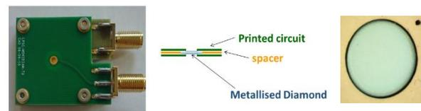
Fig. 2 The diamond sensor with a disk shaped metallization housed in its socket.
