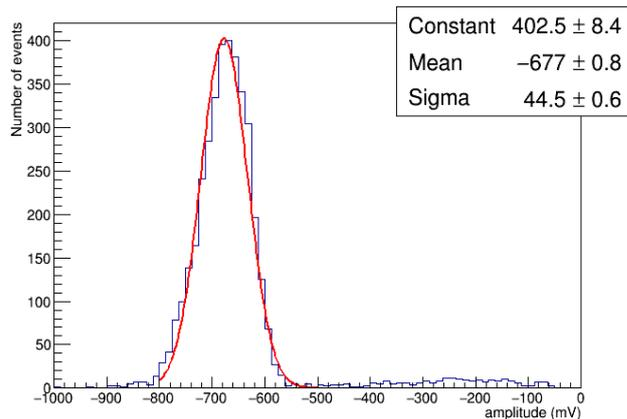
Fig. 9. Energy resolution measured on a  $0.5 \times 0.5 \text{ cm}^2 \times 300 \text{ }\mu\text{m}$  polycrystalline diamond with 95 MeV/u carbon ion beam.
