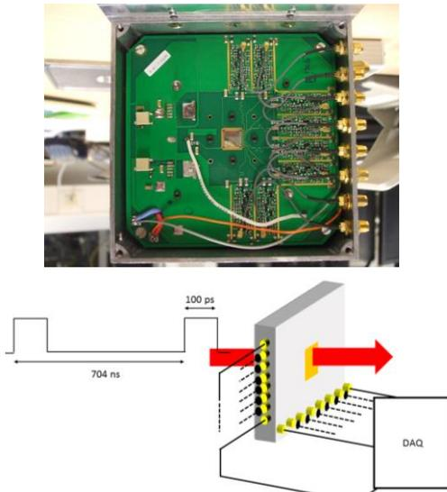
Fig. 6 ESRF experimental test bench (top : the 1 cm<sup>2</sup>, double side stripped diamond mounted on the PCB inside an electromagnetic shielding box. 8 discrete in-house preamplifiers are mounted on each side, bottom : the box positioned on the ESRF ID21 beam line).
