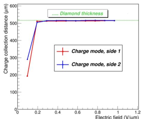
Fig. 5 The charge collection distance measured with the  $\beta$  test bench on a  $0.45 \times 0.45$  mm<sup>2</sup>  $\times$  518  $\mu$ m sCVD diamond manufactured by Element 6.
