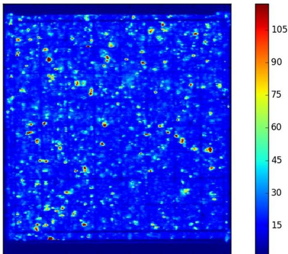
Fig. 12 X-Ray analysis of the surface of a  $10 \times 10 \text{ mm}^2 \times 300 \mu\text{m}$  double-side stripped pCVD diamond from Element 6.
