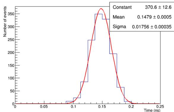
Fig. 8 Time resolution measured between a  $0.45 \times 0.45 \text{ cm}^2 \times 518 \text{ }\mu\text{m}$  sCVD diamond and a  $0.5 \times 0.5 \text{ cm}^2 \times 300 \text{ }\mu\text{m}$  DOI detector, traversed by a single carbon ion at 95 MeV/u incidence energy.
