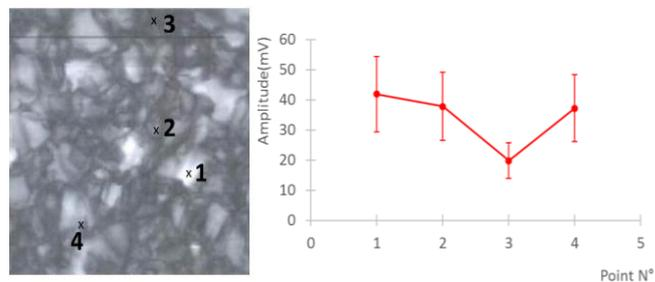
Fig. 10 Amplitude (right) of the signal versus the ESRF-ID21 pencil beam localization from point 1 up to 4 on the current-readout surface map (left) of a  $1 \text{ mm}^2$  area of a  $1 \times 1 \text{ cm}^2 \times 500 \text{ }\mu\text{m}$  polycrystalline diamond detector.
