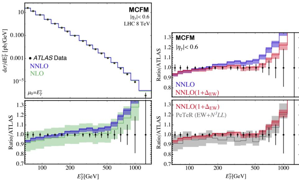
**Figure 2.** (Left) A comparison of the MCFM predictions [7] for the transverse momentum of the photon to ATLAS 8 TeV data. (Right) Upper: the effect of including electroweak corrections in addition to the NNLO predictions provided by MCFM. Lower: a comparison of the NNLO+EW prediction of MCFM with the N3LL+EW prediction of PeTeR [8].
