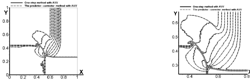
Figure 2. Isolines of density. Left: overall view. Right: enlarged view showing discontinuity interactions.
