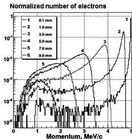
Figure 5. Momentum spectra of electrons after passing the Aluminum attenuators of different thickness. Momentum of primary electrons is 5 MeV/c
