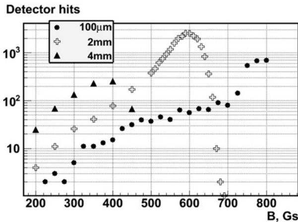
**Figure 7.** Magnetic field scans for different attenuator thickness.
