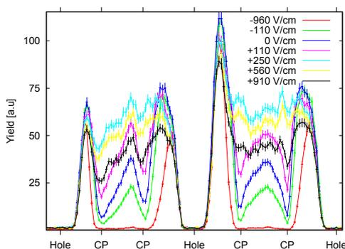
**Figure 4.** Photo-electron yield along the critical-line scans show the change of the function for several of the applied drift bias. The influence is most crucial at the critical point.
