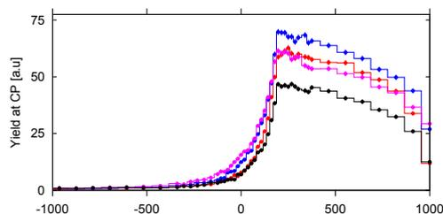
**Figure 5.** Photo-electron yield of the critical point highly depends on the applied drift field above the ThickGEM (which is responsible for the photoconversion itself).
