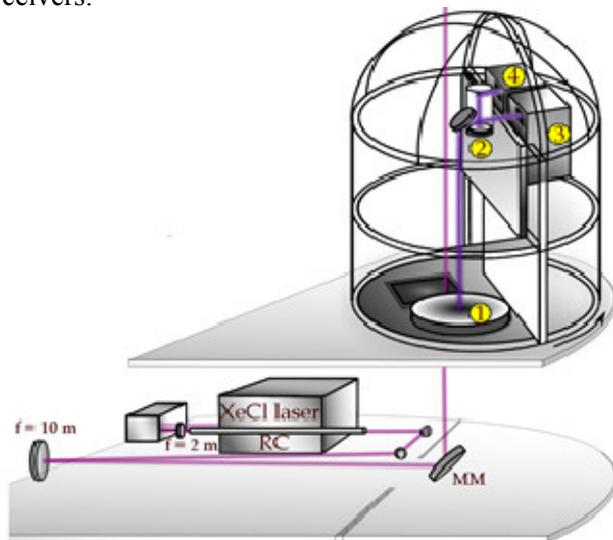
**Figure 1** (From Ref. 10) The radiation from both telescopes (1,2) is focussed into two six-channel polychromators shown in Ref. 9 (3, 4). A combination of polarization-sensitive optics and interference filters (Laseroptik G.m.b.H. and Materion Barr). The spectral widths are 0.25 nm (f.w.h.m.) for all channels except for  $\text{H}_2\text{O}$  where a 0.75-nm filter with 70 % transmittance is used. RC: Raman cell; MM: beam-steering mirror
