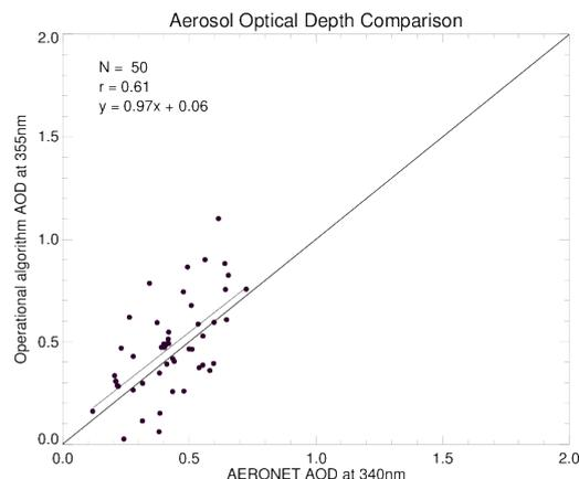
Figure 3: Comparison of the operational algorithm AOD at 355nm with the sunphotometer AOD at 340nm.
