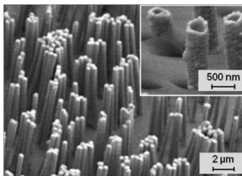
**Fig. 1.** SEM images of pristine FeNi nanotubes (nanotubes taken out from the PET templates).
