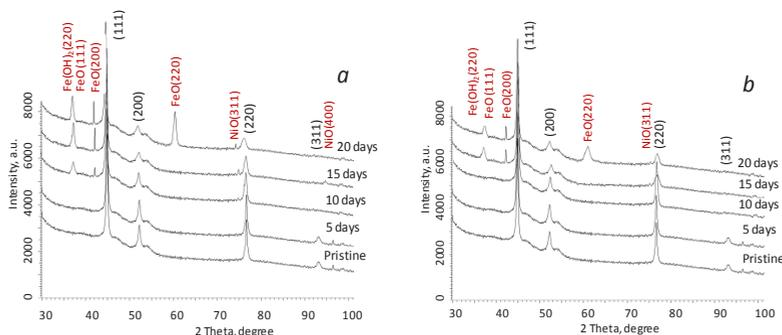
**Fig. 2.** XRD patterns of FeNi nanotubes exposed in media with various acidity: a) pH=1, b) pH=5.
