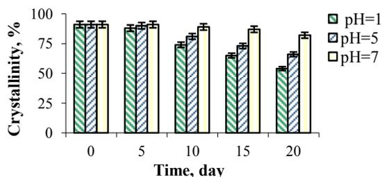
**Fig. 3.** Diagram of the changes in the FeNi nanotubes crystallinity degree exposed in media with various acidity.
