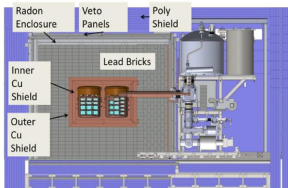
**Figure 1.** An illustration of the MAJORANA DEMONSTRATOR shield system in cross section. Detectors are denoted by blue disks stacked in strings installed in two electroformed copper cryostats. The cryostats are surrounded by electroformed inner- and clean-commercial outer copper shields. Lead bricks, a radon enclosure, muon veto panels, and polyethylene shields complete the shield system.
