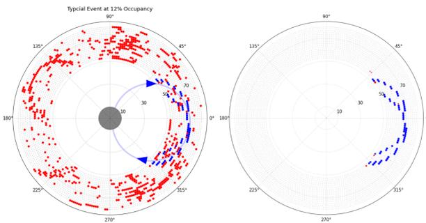
**Figure 3.** Reconstruction of simulated tracks. In the first step [left] hits are classified as signal-like (blue) or background-like (red). In the second step [right], a Hough transform based on the signal-like hits is used to select hits belonging to a track, which can be reconstructed in 3D using the two stereo projections.
