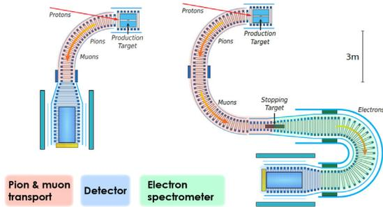
**Figure 2.** Plan view of Phase-I [left] and Phase-II [right] of COMET. The Capture section and first 90° are common to both Phases.
