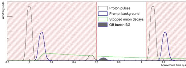
**Figure 1.** Cartoon of the delayed window technique. The prompt backgrounds (blue) should all occur a few hundred nanoseconds after the primary beam time, while the signal occurs according to the lifetime of the muonic atoms, which is matched to the bunch frequency. An important aspect is whether there are non-negligible off-time bunches (grey fill). In reality, such a background is not expected to be a problem, as described in the next section.
