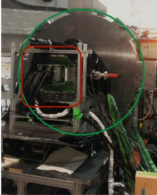
**Figure 4.** The test-beam prototype Phase-II detector, during the run at ELPH. The Straw Tube Tracker and Calorimeter pieces are indicated in green and red respectively.
