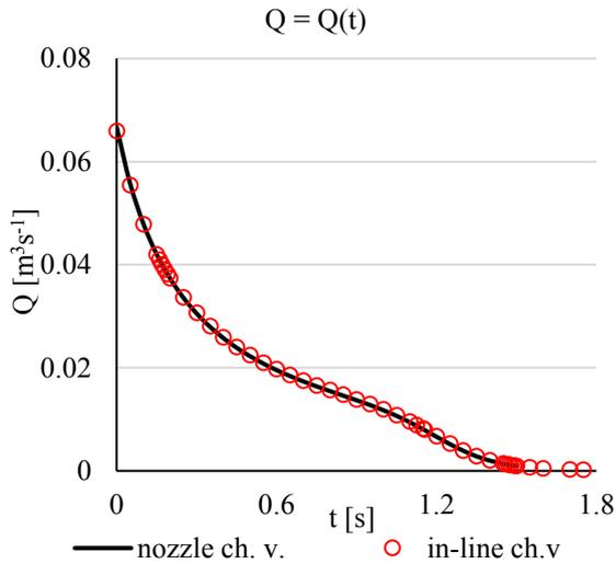
**Fig. 8.** 1AM simulations of the in-line and nozzle check valve in the piping system, the flow rate.
