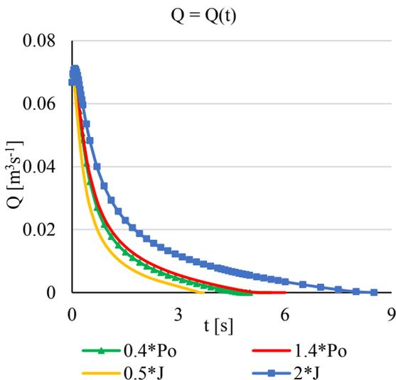
Fig. 13. 1DOF CFD and 1AM simulations of the in-line check valve, the flow rate.
