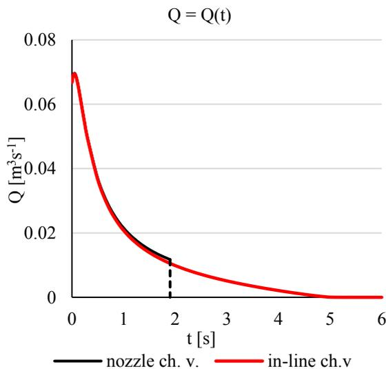
**Fig. 10.** 1AM in-line valve and nozzle check valve simulations in the piping system in case of a sudden failure of centrifugal pump during a power outage, the flow rate.
