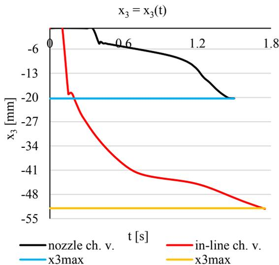
**Fig. 9.** 1AM simulations of the in-line and nozzle check valve in the piping system, the disc and the poppet positions.
