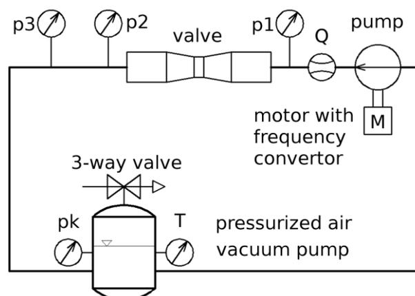
**Fig. 3.** The pipeline and the testing circuit diagram
