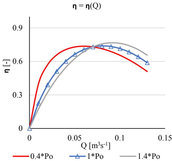
Fig. 12. The pump efficiency curves.
