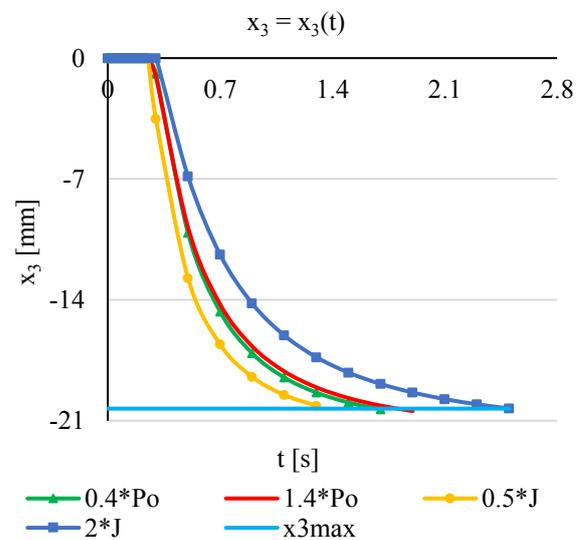
Fig. 16. 1DOF CFD and 1AM simulations of the nozzle check valve, the positions of the disc.
