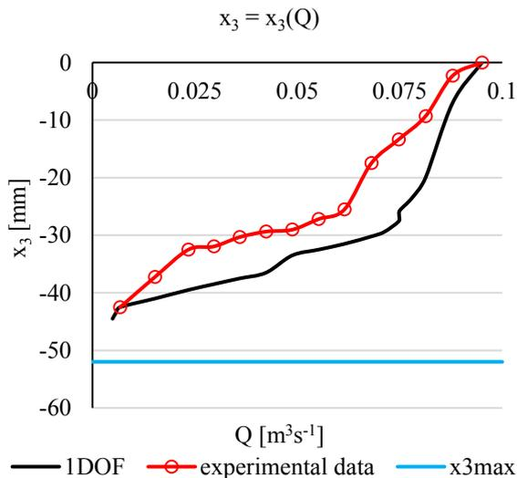
**Fig. 5.** 1DOF CFD In-line check valve simulation and comparison with experimental data,  $T_s = 1.5s$ .
