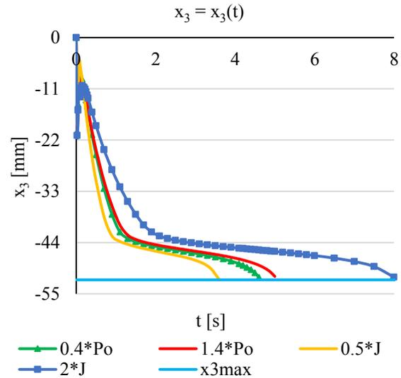
Fig. 14. 1DOF CFD and 1AM simulations of the in-line check valve, the positions of the poppet.
