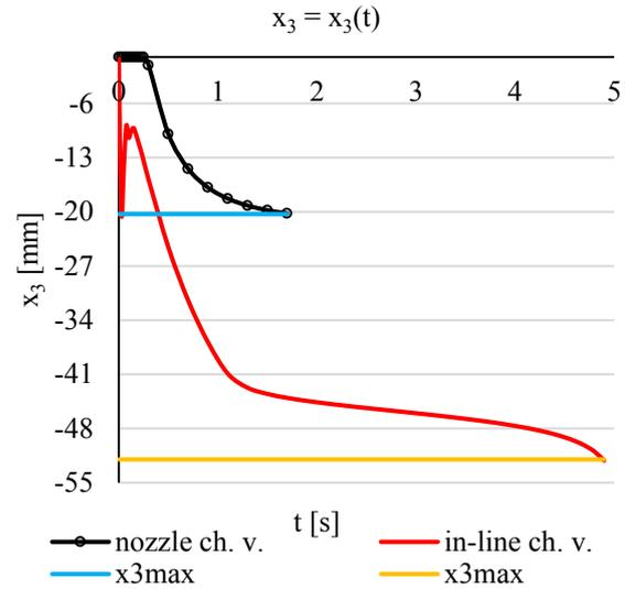
**Fig. 11.** 1AM in-line valve and nozzle check valve simulations in the piping system in case of a sudden failure of centrifugal pump during a power outage, the disc and the poppet positions.
