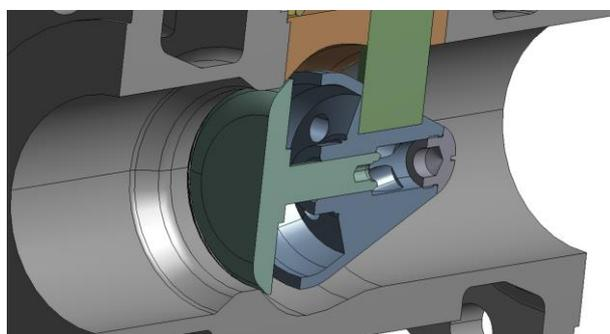
**Fig. 1.** Nozzle check valve.
