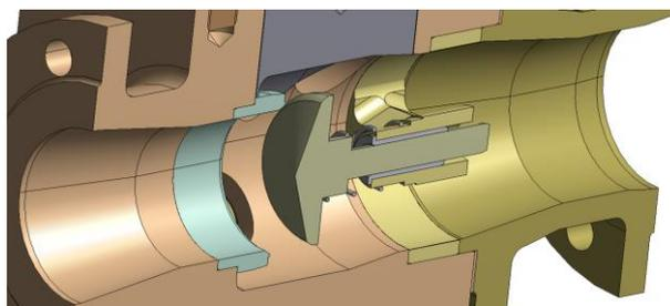
**Fig. 2.** In-line check valve.
