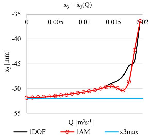
**Fig. 6.** 1DOF CFD and 1AM in-line valve simulations,  $T_s = 0.5s$  and initial opening 30%.
