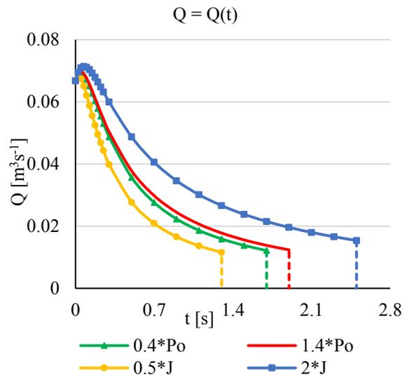
Fig. 15. 1DOF CFD and 1AM simulations of the nozzle check valve, the flow rate.
