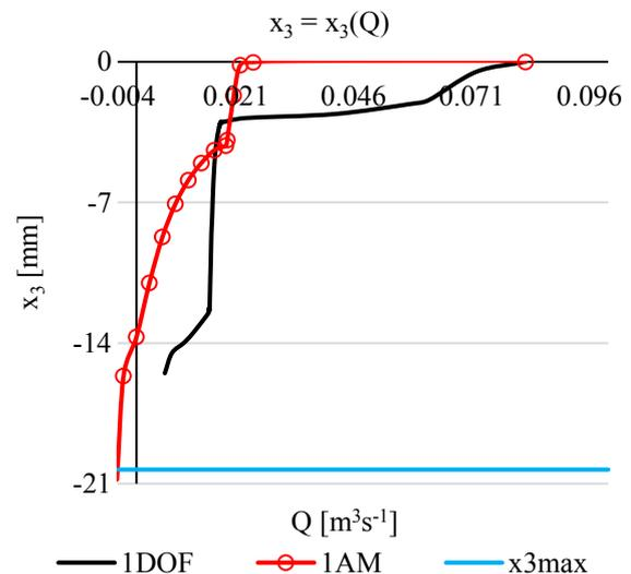
**Fig. 7.** 1DOF CFD and 1AM simulations of the disc position of the nozzle check valve,  $T_s = 1.5s$ .
