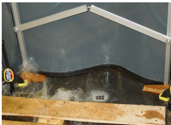
Fig. 5. Experimental measurement: hydrodynamic load of anti-flood board
