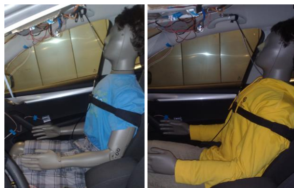
Fig. 1. Thermal manikin with summer and winter clothing.
