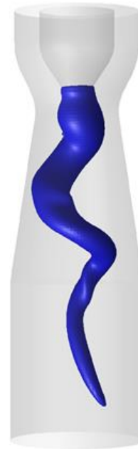
Fig. 8. Snapshot of the instantaneous pressure field visualizing the pressure contour of the vortex rope
