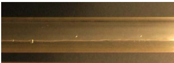
Fig. 2. Fragment of a large bubble entrusts resulting from the slug flow.
