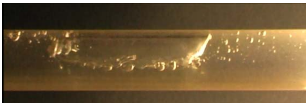
Fig. 3. Small bubble formed in the slug flow.
