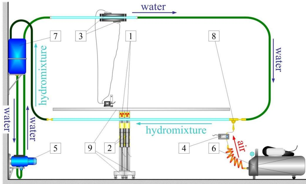
**Fig. 1.** Schema of laboratory experimental set-up: 1 –sealed Am-241 sources with collimators, 2 – scintillation probes, 3 – ultrasonic flow meter of water, 4 – mass flow meter of air, 5 – pump with power inverter, 6 – compressor 50l, 7 – expansion tank, 8 – injector, 9 – shift system.
