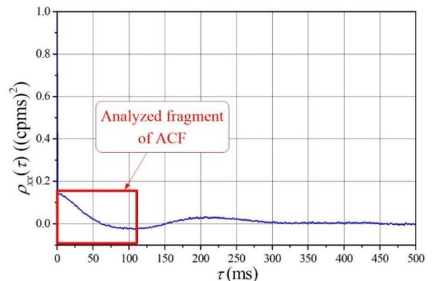
**Fig. 2.** Exemplary plot of ACF obtained in the selected experiment. Red frame indicated the fragment which is related to the change of air velocity.
