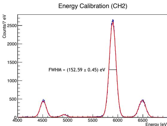
**Figure 3.** Energy calibration of one SDD channel (channel 2) obtained with a Fe-55 source and an additional Ti foil.
