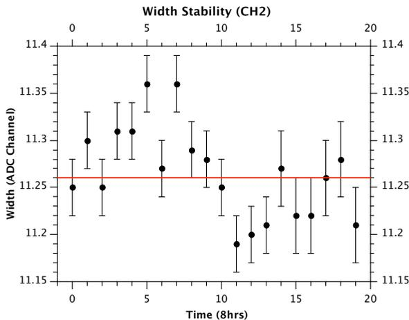
**Figure 5.** Width Stability of the Mn  $K_{\alpha}$  width of one SDD channel (channel 2). The red line indicates the average width of the data sample corresponding to 148.0 eV with fluctuations of  $\pm 1.0$  eV.
