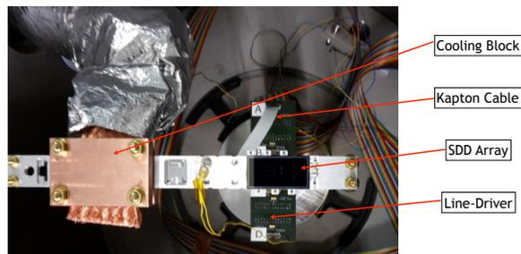
**Figure 2.** Test setup of the E57 experiment at the Stefan Meyer Institute including the cooling block, one single SDD array and the line-driver
