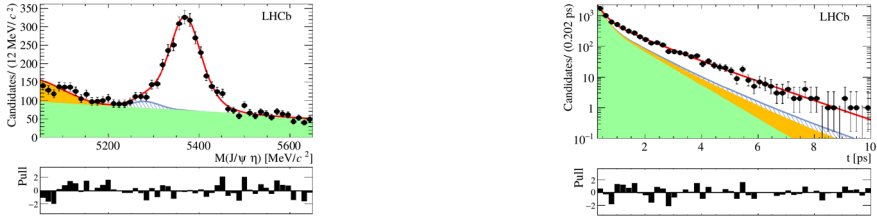
Figure 8. Distributions of J/\psi\eta invariant mass and decay time for selected B_s^0 \rightarrow J/\psi\eta decays. Combinatorial background (green), background from B^0 \rightarrow J/\psi\eta decays (blue) and partially reconstructed background (orange) are shown.
