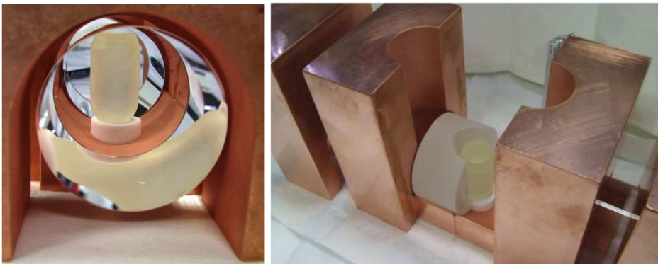
Figure 2. Pictures of the ^{106}\text{CdWO}_4 set-up during the assembling. On the left: the ^{106}\text{CdWO}_4 installed in the central part of the set-up. On the right: one of the \text{CdWO}_4 enclosing the enriched scintillator is shown together with some copper shaped bricks.
