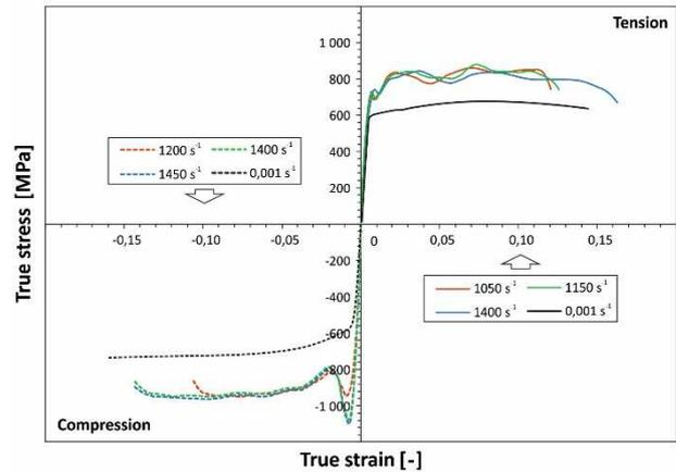
**Fig. 5.** Stress-strain curves in tension and in compression for B500A steel.
