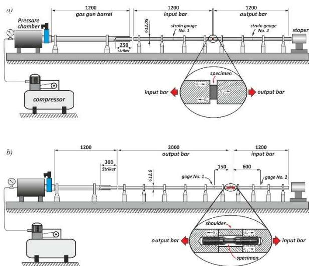
**Fig. 2.** Hopkinson bar technique apparatus is used to investigate the dynamic behaviours of tested steels in compression (a) and tension (b).
