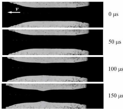
**Fig. 3.** Selected high-speed camera images showing the specimen tension made of B500A steel.
