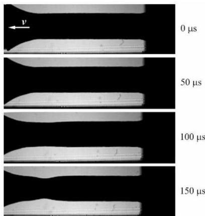
**Fig. 4.** Selected high-speed camera images showing the specimen tension made of RB500W steel.
