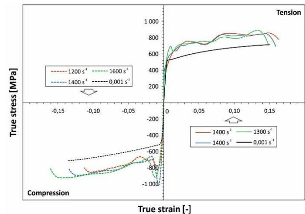
**Fig. 6.** Stress-strain curves in tension and in compression for RB500W steel.
