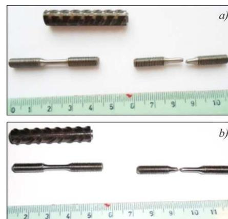
**Fig. 1.** General views of sections of rebar steels tested, as well as tensile specimens before and after tests. a) B500A, b) RB500W.
