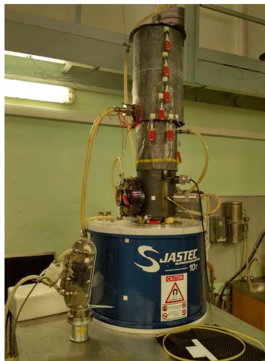
Fig. 1. The general view of the 250 GHz gyrotron installed in the cryomagnet
