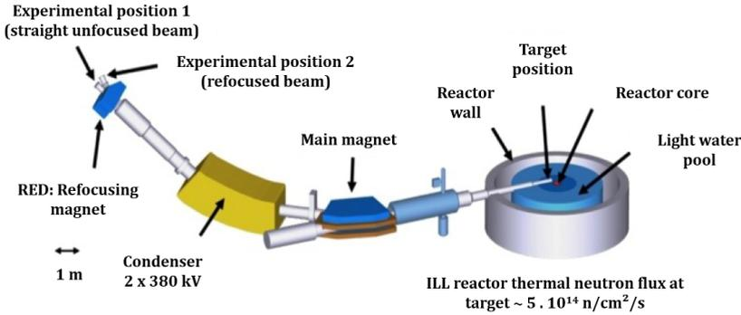
**Figure 1.** Lohengrin mass spectrometer at the ILL, Grenoble. The ILL high neutron flux compensates the small geometrical acceptance of the instrument.
