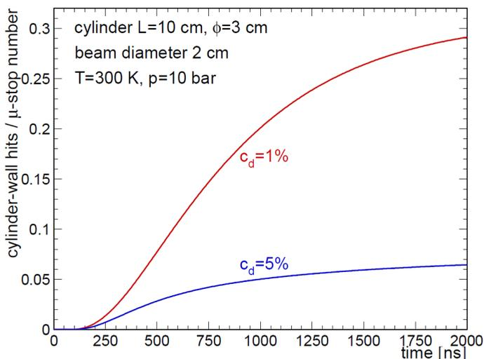
**Figure 1.** Time-dependent total integrated probability (per stopped muon) that the  $\mu\text{D}$  atoms hit the walls of a cylindrical volume with length  $L$  and diameter  $\phi$ . The red curve and the blue curves show the calculation for a deuterium concentration  $c_d$  of 1% and 5%, respectively.
