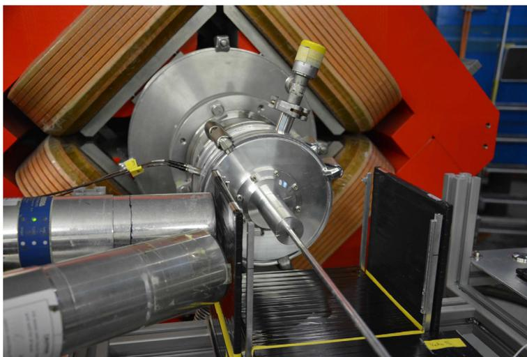
**Figure 3.** Room temperature hydrogen cell mounted at the end of the  $\pi$ E5 beam line. The last quadrupole magnet of the beam line is visible. The cell was operated routinely at 10 bar hydrogen/deuterium mixtures. A plastic scintillator (in vacuum) was mounted in the beam line in front of the gas cell.
