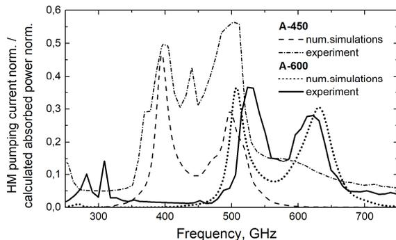
**Fig. 3.** Experimental results of HM pumping by FFO power and calculation results of the absorbed FFO power by HM. The HM pumping current is normalized to the “current jump” at the gap SIS voltage. The absorbed power is normalized to the total output FFO power.
