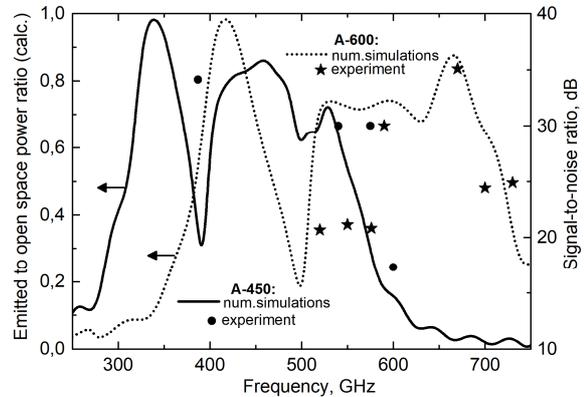
**Fig. 4.** Calculation results of power emitted by antenna to open space normalized to the total output FFO power (left axis); experimental points of output emission detected by SISP at some frequencies (right axis).
