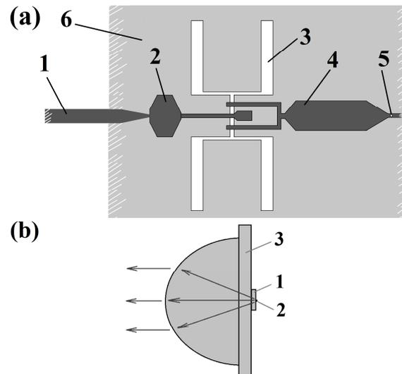
**Fig. 1.** (a) layout of the planar structure of THz oscillator (1) based on a long SIS junction coupled by microstrip line (2) to slot antenna (3) and by microstrip line (4) to harmonic SIS mixer (5), metallization layer (6) of antenna is also the bottom electrode of the microstrip and the SIS junctions; (b) scheme of the chip (1) with oscillator and antenna shown on (a) placed at the far focus (2) of the silicon lens (3). The scheme (b) is not to scale.
