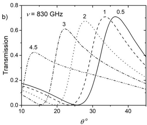
**Fig. 3.** PMS transmission at 830 GHz as the function of the incident angle  $\theta$  modelled for different thicknesses  $d$  of the analyte overlayer. The numbers indicate the values of  $d$  in micrometers.
