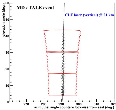
**Figure 2.** Event display of a CLF laser shot as recorded by the MD/TALE FDs. Two MD, and one TALE telescopes (mirrors) participate in the event, mirror boundaries shown in red. The track starts at the bottom of the lowest elevation viewing mirror.
