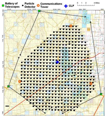
**Figure 1.** Map of the Telescope Array surface detector and the three fluorescence detectors overlooking the array. The CLF location is indicated by the blue “+” at the center of the SD array. The green squares mark the locations of the three FD stations: Black Rock (BR) near bottom right, Long Ridge (LR) near bottom right, and Middle Drum (MD) near top of figure.
