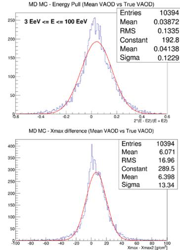
**Figure 5.** Energy and  $X_{max}$  Pull: Mean VAOD vs MC thrown “true” parameters.
